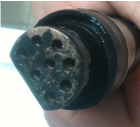
Figure: Corrosion visible on the female Burton connector following deployment and camera failure.
