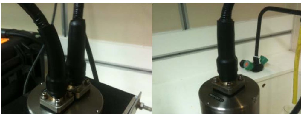
Figure: initial attempts to seal Burton connectors.
