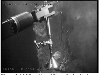
**Figure 2.4.5.2** Sampling of Sisters Peak with the IB-sampler
