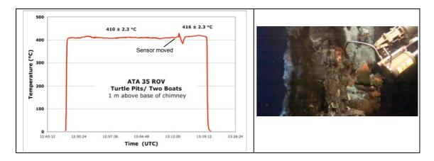
**Fig. 2.4.4.3:** Station ATA 35 ROV, Turtle Pits. Temperature readings and fluid sampling was at a small outlet approx. 1m above the base of Two Boats. Average over 20 minutes:  $410 \pm 2.3$  °C. After the sensor had been repositioned temperature readings were  $416 \pm 2.3$  °C over 5 minutes. The maximum temperature recorded was  $T_{max} = 429$  °C. KIPS fluid sampling failed. Ti Major D2 filled, 35 ROV-7.
