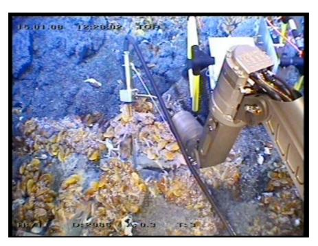
Fig. 2.4.3.2: Measurment of temperature with the 8-channel temperature logger at the low-temperature diffuse outlet at Wideawake (37 ROV6).
