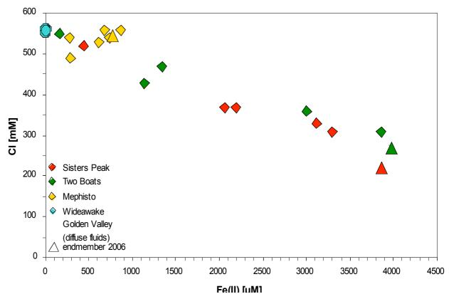
Fig. 2.4.4.11: Crossplot of Fe(II) and Cl concentrations for hot and diffuse hydrothermal fluids
