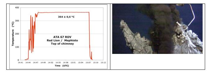
**Fig. 2.4.4.9:** Station ATA 67 ROV, Red Lion. A newly opened orifice in the summit region of the Mephisto chimney was sampled with Ti Major D2, 67 ROV-3, and KIPS fluid samples 67 ROV-4 to -8. Clear fluid was leaving the outlet of KIPS. Temperatures were  $364 \pm 0.6$  °C with a maximum of 366 °C.
