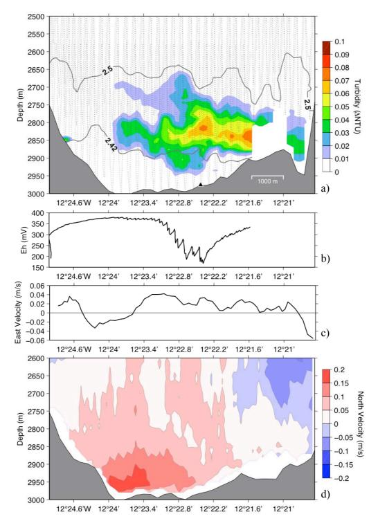
Fig. 2.4.1.6 Observations during a 5 nm long tow-yo crossing the rift valley from west to east. The CTD was navigated using POSIDONIA. (a) Turbidity from three MAPRs, one mounted on the CTD frame and two attached to the wire 100 m and 200 m above the CTD. (b) Eh from the MAPR parallel to the CTD. (c) Mean eastward current velocity below 2750 m from ADCP measurements. (d) Contours of northward velocity from ADCP measurements.
