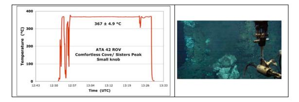
**Fig. 2.4.4.6:** Station ATA 42 ROV, Comfortless Cove. Temperature readings and fluid sampling were at a small knob in the top region of the Sisters Peak chimney. Average over 20 minutes:  $367 \pm 4.9$  °C,  $T_{max} = 379$  °C, KIPS fluid samples 42 ROV-2 to -5 taken and Ti-Major D1 42-ROV-7 filled. KIPS fluid samples 42 ROV-11 to -14 were taken without temperature reading because the cable had been cut during handling.
