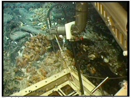
Fig. 2.4.3.6: Measurment of temperature with the 8-channel temperature logger at the low-temperature diffuse outlet at Clueless (52 ROV10).
