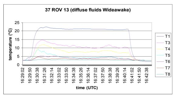
Fig. 2.4.3.5: Measurment of temperature with the 8-channel temperature logger at the low-temperature diffuse outlet at Wideawake (37 ROV13). T1 = 28 cm depth, T3 = 24 cm, T4 = 20 cm, T5 = 16 cm, T6 = 12 cm and T7 = 8 cm.
