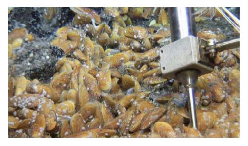
Fig. 2.4.3.4: Measurment of temperature with the 8-channel temperature logger at the low-temperature diffuse outlet at Wideawake (37 ROV13).
