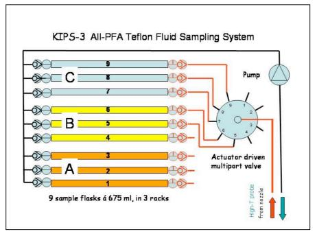
**Fig. 2.4.4.1:** Schematic configuration of the inert KIPS fluid sampling system (only tubing connections to flasks # 5 - # 9 are shown for clarity). Fluid entering the nozzle is distributed by a motorized multiport-valve to 9 PFA sample flasks á 675 ml, each with check valves and stopcocks. The pump is positioned downstream. Racks A, B, C with 3 flasks each can be quickly removed and sub-sampled in the lab.
