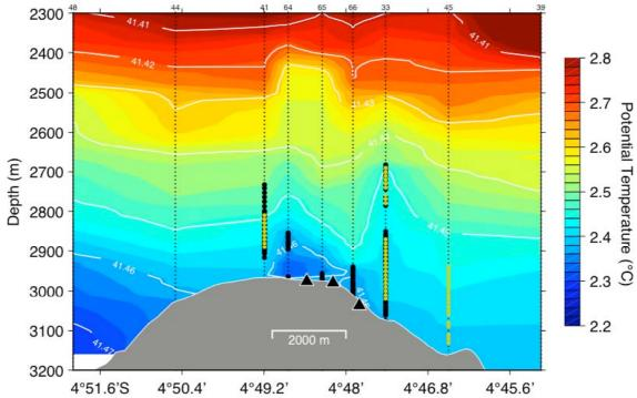
Fig. 2.4.1.2 Potential temperature section along the rift valley put together from nine non-synoptic CTD stations. Contours of potential density ( $\sigma_3$ ) are shown in white. Transmission and Eh anomalies are marked with yellow and black dots (no Eh data on station 45). The locations of the vents sites are indicated by black triangles.
