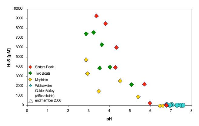
Fig. 2.4.4.12: Crossplot of pH and  $H_2S$  concentrations for hot and diffuse hydrothermal fluids
