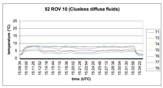
Fig. 2.4.3.7: Measurement of temperature with the 8-channel temperature logger at the low-temperature diffuse outlet at Clueless (52 ROV10). T1 = 28 cm depth, T3 = 24 cm, T4 = 20 cm, T5 = 16 cm, T6 = 12 cm and T7 = 8 cm.
