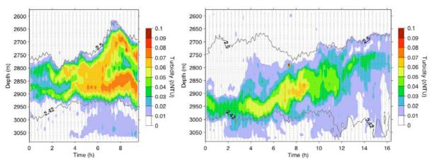
Fig. 2.4.1.4: Time series of turbidity measured during two yoyo stations carried out on January 14/15 (left) and January 22/23 (right), both at the same location about 700 m north of the Red Lion vent field (at station 33 in Fig. 2.4.1.1). Also shown are two temperature contours, that depict the upper and lower boundaries of the non-buoyant plume.
