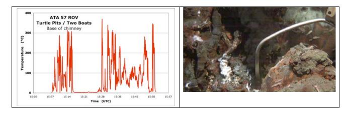
**Fig. 2.4.4.8:** Station ATA 57 ROV, Turtle Pits. KIPS fluid samples 57 ROV-2 to -5 collected again at base of chimney Two Boats. The orifice was now even more plumbed, and fluid flow was significantly reduced. Every attempt to reopen the orifice failed. The maximum temperature reading was 371 °C.
