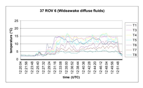
Fig. 2.4.3.3: Measurment of temperature with the 8-channel temperature logger at the low-temperature diffuse outlet at Wideawake (37 ROV6). T1 = 28 cm depth, T3 = 24 cm, T4 = 20 cm, T5 = 16 cm, T6 = 12 cm and T7 = 8 cm.
