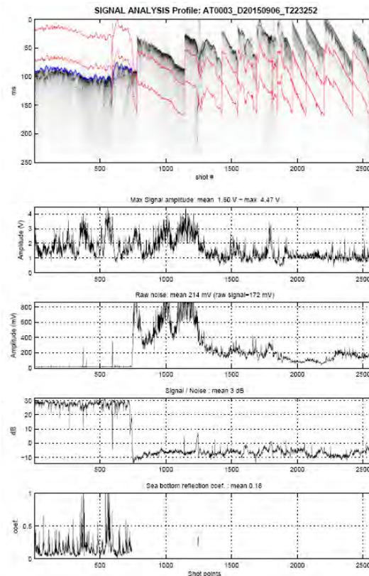
**Figure 35 - Example of error in seafloor detection : the start of the profile uses a correct value for the water depth. Starting from shot point 750, the acquisition window is too deep, leading to occasional data loss of the seafloor reflector, and erroneous calculation of the signal to noise ratio.**
