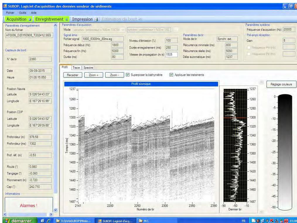
Figure 30 – Screenshot of the SUBOP acquisition system visualization, showing real time images of the sub-bottom profiler data acquisition
