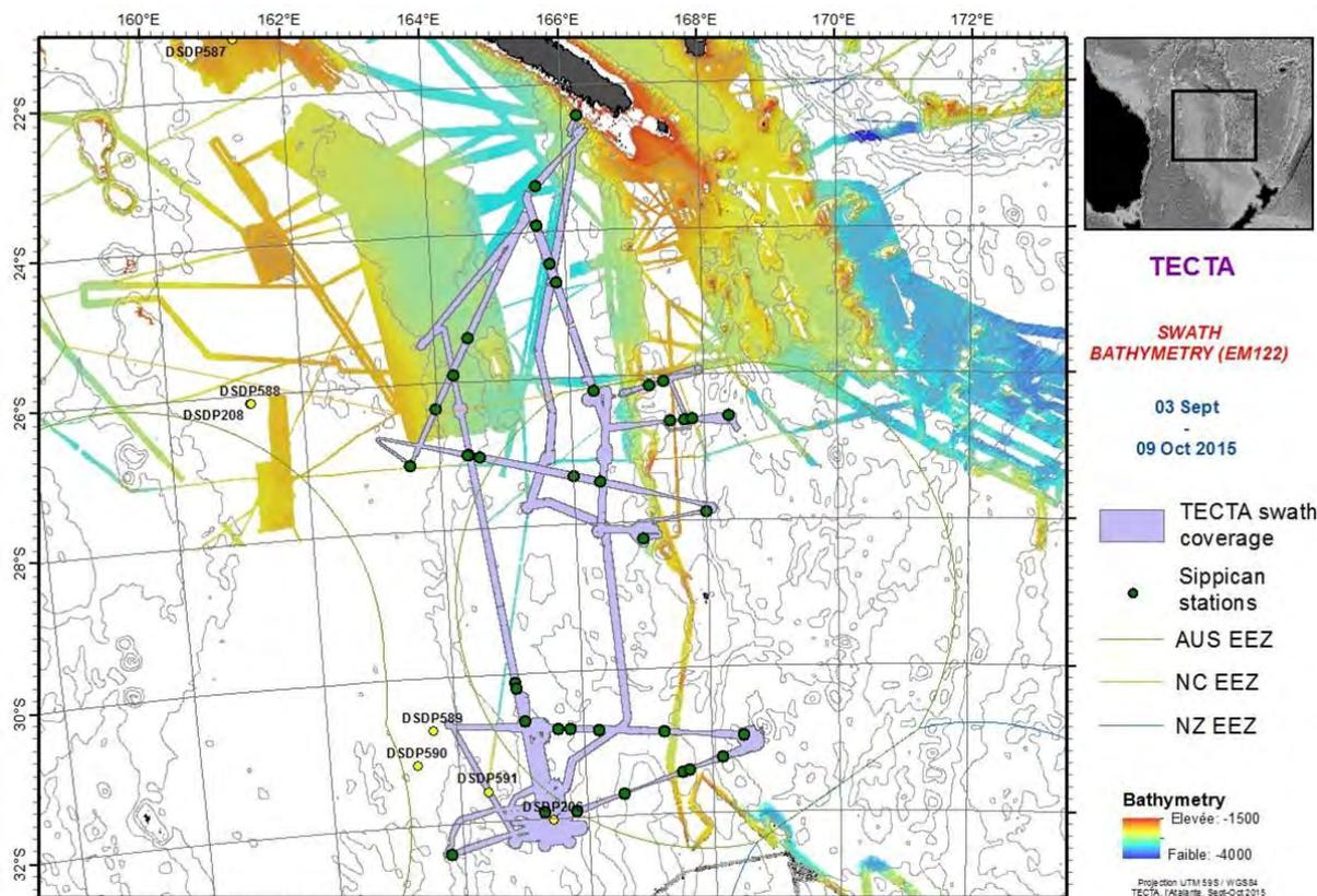
Figure 12 – Map showing the location of deployment of XBT probes, TECTA swath coverage and existing swath data.
