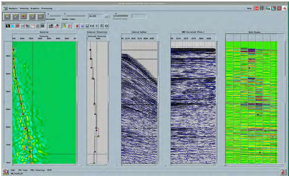
Figure 27 – Example of velocity picking panel with semblance in Geocluster
