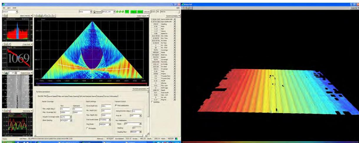
Figure 13 – Screen shot of the SIS acquisition visualization system, showing real time images of the multi-beam echo sounder data acquired by the EM122 system. Sediment waves are visible in this image.
