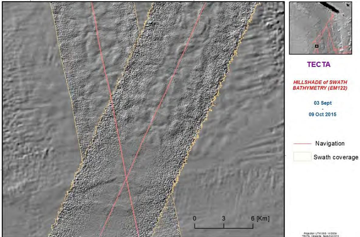
**Figure 14 – Crossing of bathymetric profiles revealing noisy outer beams. Background is EM12 data from Zonoco05 voyage (1999).**
