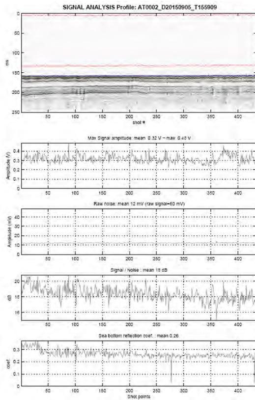
**Figure 36- Example of Subop acquisition window starting too early. The result is that only about 90 ms of useful data are acquired, which is significantly less than the maximum penetration in this particular area.**
