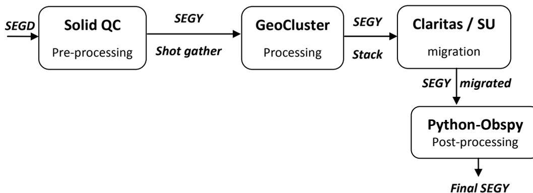
**Figure 23 - Summary of seismic processing sequence**
