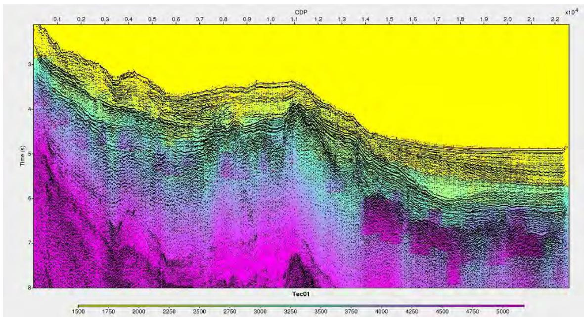
Figure 28 – Time migrated section of profile TEC001 with stacking velocities superimposed.
