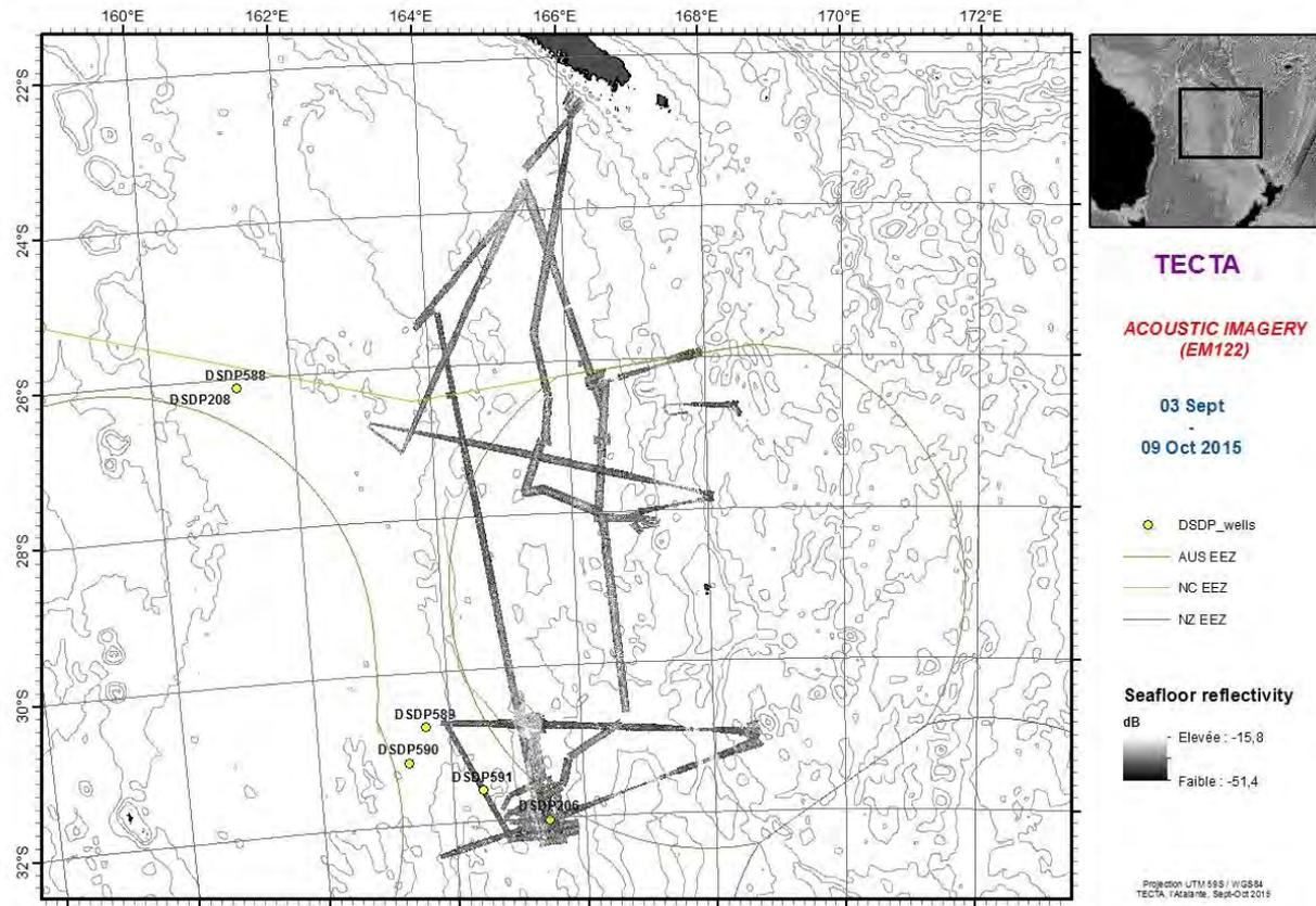
Figure 19 Acoustic imagery data acquired during the TECTA voyage
