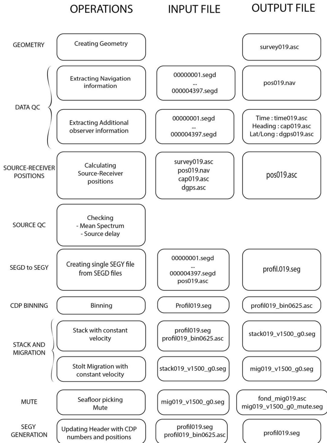
**Figure 24 - Processing steps in Solid QC-, input and output files generated.**
