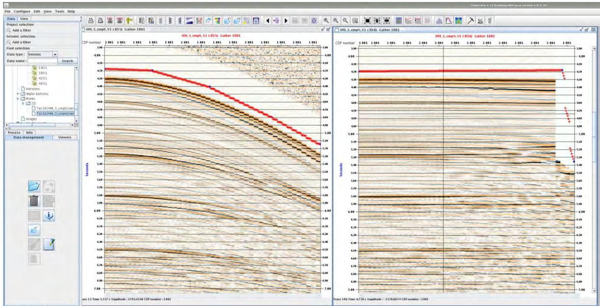
Figure 26 – Example of sea floor mute from uncorrected and NMO corrected data
