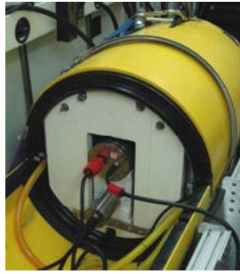
Fig. 11: Methane sensor fitted into the AWI AUV. The sensor was connected in series with a pumped conductivity sensor (CTD) leading the ambient water through both sensors (left, middle). Unfortunately, bad weather and sea conditions prohibited the deployment of the AUV at the Håkon Mosby Mud Volcano. The only trial that was possible had to be aborted due to rapidly increasing winds and high swell during the dive of the AUV (right).
