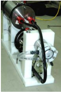
Fig. 11: Methane sensor fitted into the AWI AUV. The sensor was connected in series with a pumped conductivity sensor (CTD) leading the ambient water through both sensors (left, middle). Unfortunately, bad weather and sea conditions prohibited the deployment of the AUV at the Håkon Mosby Mud Volcano. The only trial that was possible had to be aborted due to rapidly increasing winds and high swell during the dive of the AUV (right).
