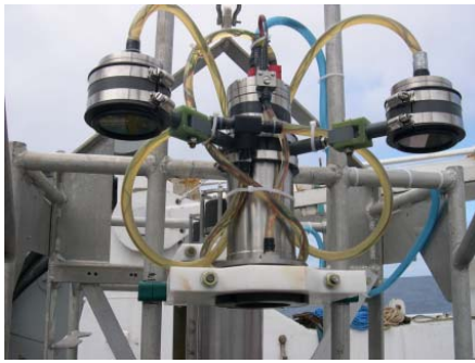
Fig. 3: MOB 0, detail of the digital still camera and of the two LED recover projectors.
