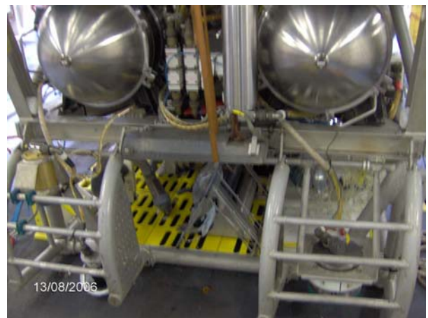
Fig.10: The DPA system is mounted in horizontal position, inside its mooring frame in Victor's toolsled
