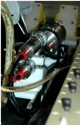
Fig. 12: Methane sensors installed in Victor 6000's survey module (left). They are in line with the newly developed water sampler PEPITO allowing a direct comparison of sensor signals and water sample methane measurements. Right: The power supply of the autonomous methanol module.
