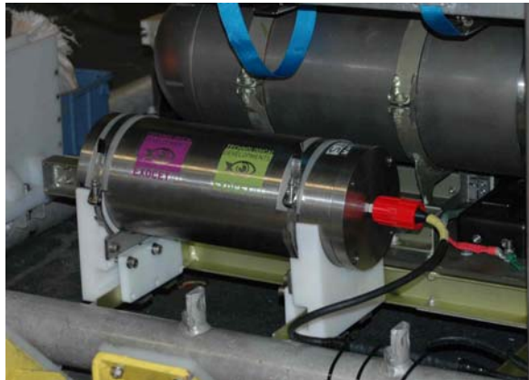
Fig. 12: Methane sensors installed in Victor 6000's survey module (left). They are in line with the newly developed water sampler PEPITO allowing a direct comparison of sensor signals and water sample methane measurements. Right: The power supply of the autonomous methanol module.
