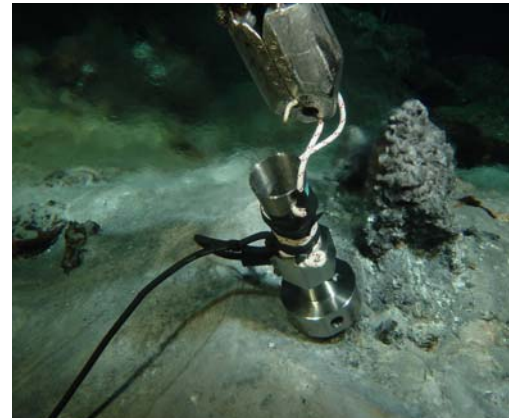
Fig.13: Fluid flow measurements on a small vent diffusing a translucent hot fluid, Menez Gwen field,
