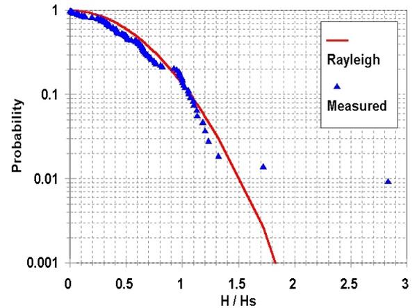
Figure 2. Wave heights compared to the Rayleigh distribution for time series in Figure 1c.
