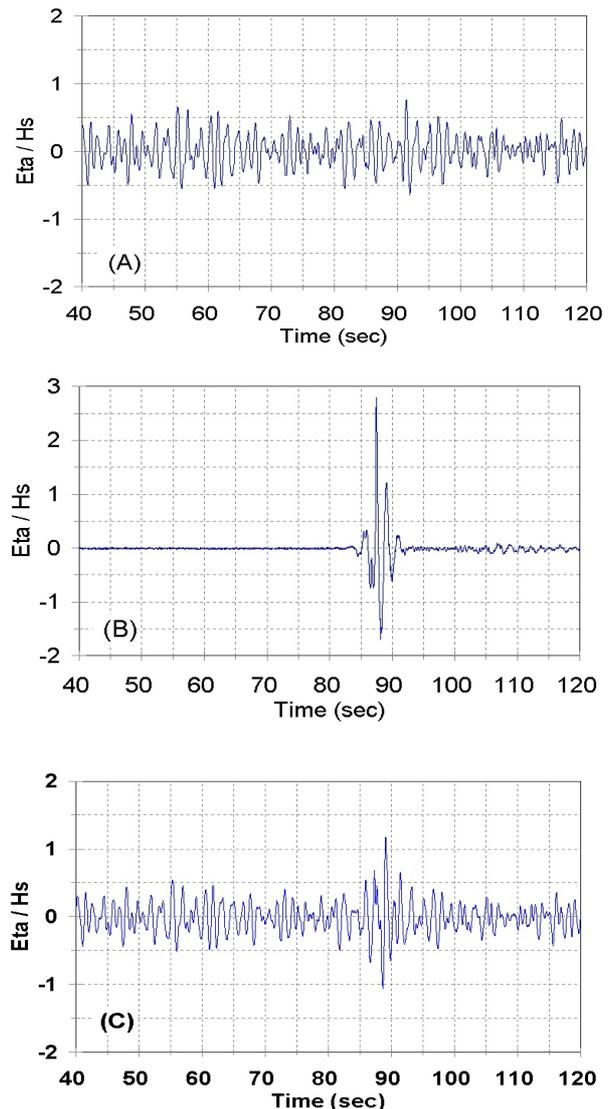
Figure 1. Sample wave records generated from the same spectrum using (a) random phases, (b) contrived phases to produce a transient wave, and (c) both contrived and random phases (20% of the energy into the transient wave and 80% into the random sea)
