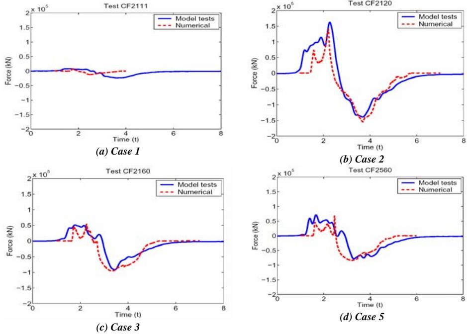
**Fig. 4.** Vertical impact force time series: comparisons between numerical results (dashed lines) and experimental results (solid lines).
