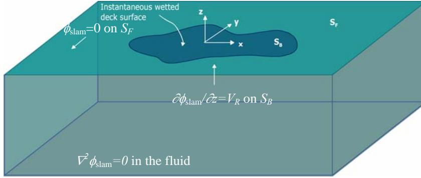
**Fig. 1.** Simplified hydrodynamic boundary value problem of the wave-in-deck event.  $\phi_{slam}$  is the impact induced velocity potential and  $V_R$  is the averaged relative impact velocity over the wetted deck area.
