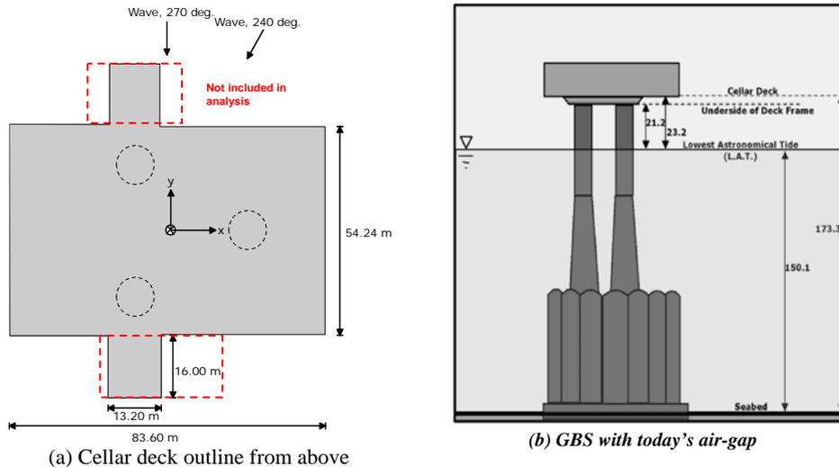
**Fig. 2. GBS model with simplified topside (from [1])**
