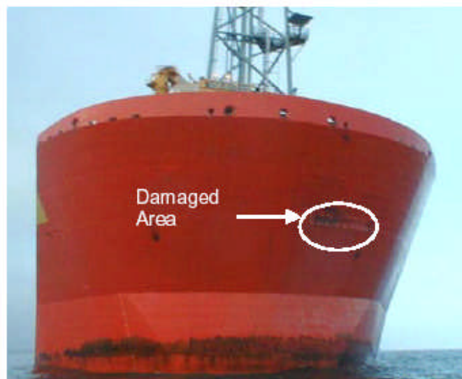
Figure 1: Damage to the Schiehallion bow
