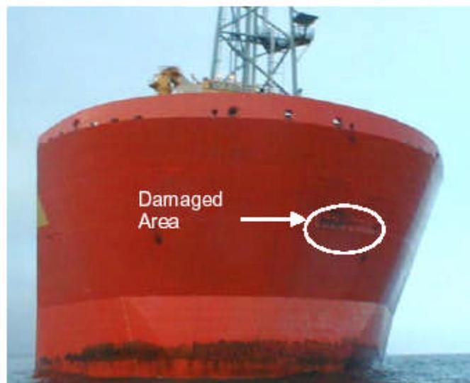
Figure 1: Damage to the Schiehallion bow
