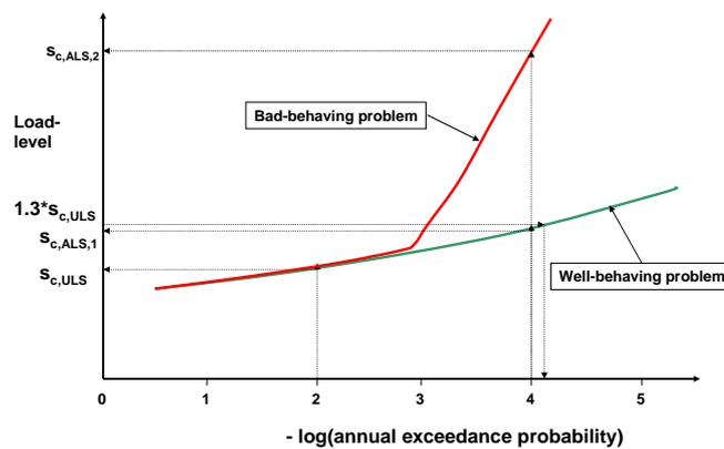
**Fig. 1.** Illustration of well-behaving and bad-behaving response problem.
