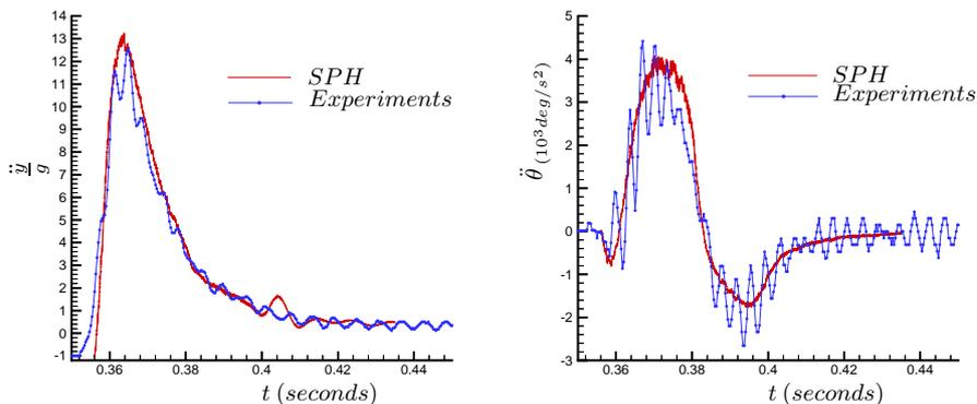
Figure 1: *Temporal evolution of the wedge vertical and angular accelerations*
