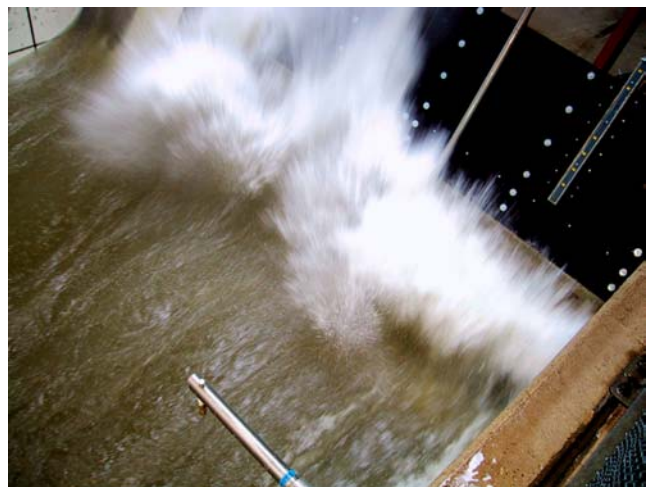
Figure 1. Wave impact on a wall sloping at 27° to the vertical. Spray caused by air escaping from a trapped air pocket at high pressure can be seen. The exposure time is 1/125 second, and the width of the flume (GWK) is 5 metres.
