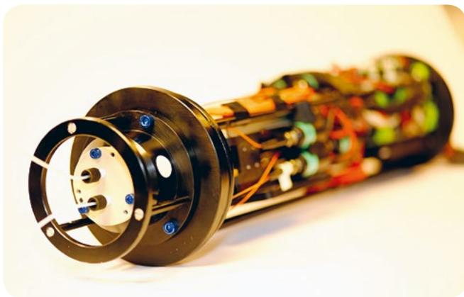
THE NEW SPRI SENSOR DEVELOPED BY IFREMER IS DESIGNED TO DETECT BIOTOXINS LIKE DOMOIC ACID IN THE OCEAN. © Ifremer
