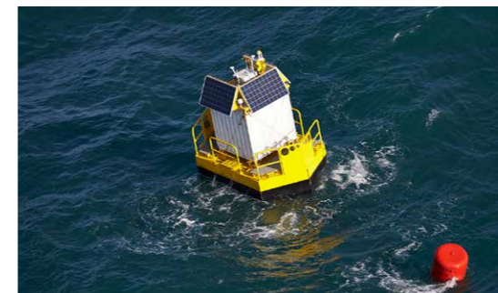
Wavepearl autonomous buoy Solar + wave energy, battery storage + monitoring instruments
